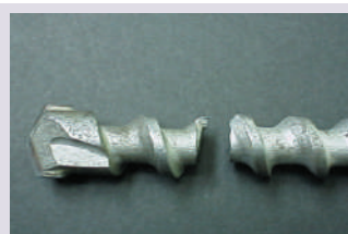
Carbide tip worn out
