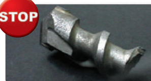
Carbide tip worn out
