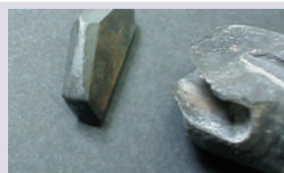
Carbide tip worn out
