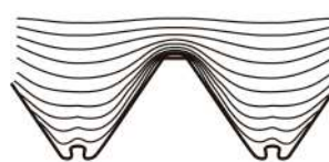
Thread obtained with a forming tap
