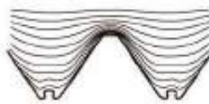
Thread obtained with a forming tap
