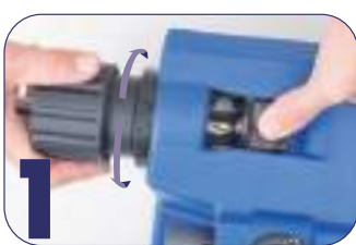
1 Place and adjust the drill in the chuck
